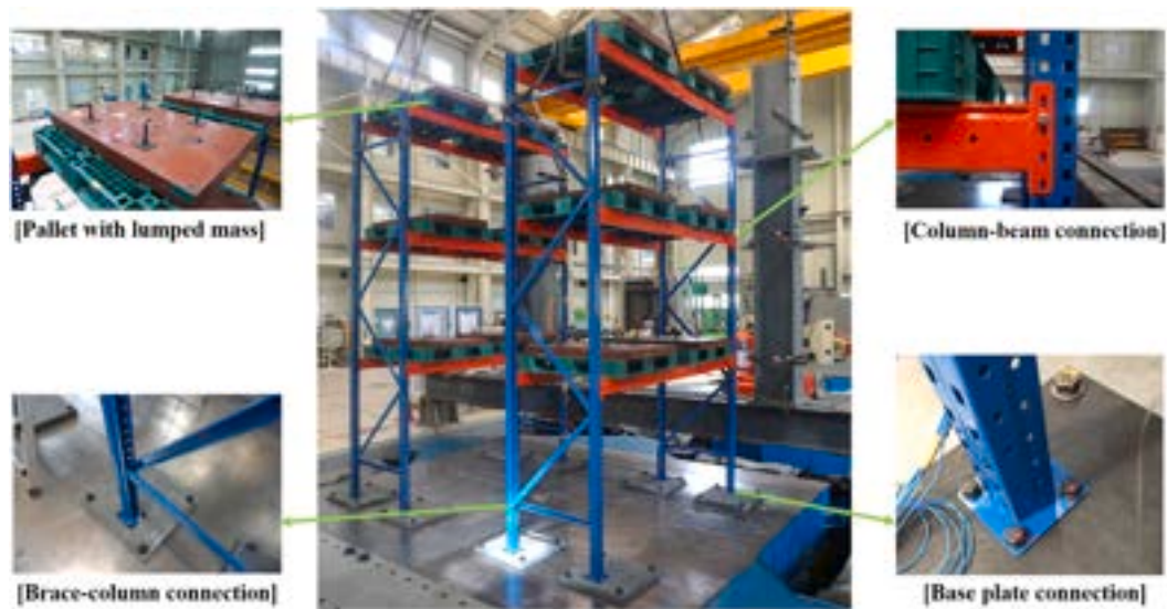
Fig. 2. Shake table test for pallet rack collapse and damage.
