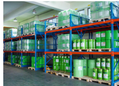
Fig. 2. Case of steel storage racks installation for storing chemical drums [23]
